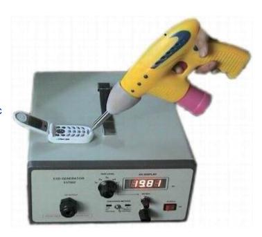
continuous adjusted electrostatic discharge pulses voltage from 0 to  $\pm 20$ KV in both air and contact discharge operations. Exceeding industry ESD test standards requiring pulse voltages of 8kv (contact)/15 kV(air). Basic model is supplied with 150 pF/330 ohm network in compliance with IEC/EN 61000-4-2,IEC 1000-4-2 and IEC 801-2 / 1991, and other optional extra discharge networks is available
